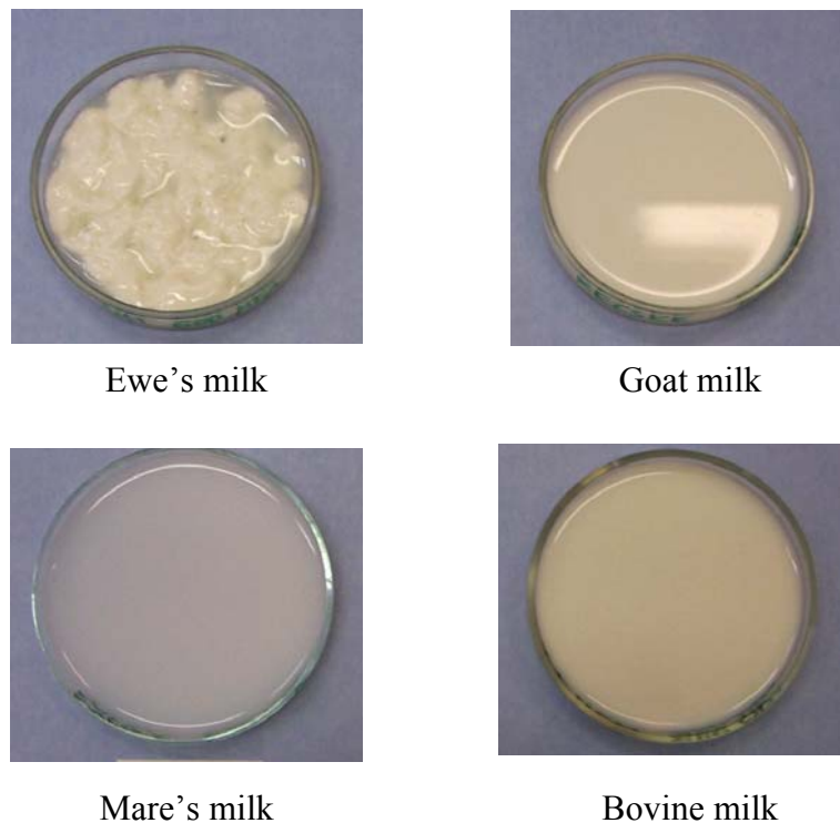
Figure 23. Photos of different milk types treated at 600 MPa for 5 mins (Photo: Dalmadi)
