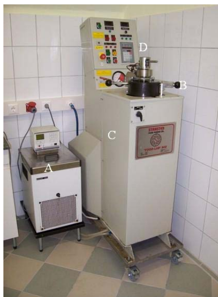
Figure 12. Food Lab® high pressure food processor; A: External cooling system; B: high lift loading system to chamber; C: rack for pump and intensifier; D: control panel.
