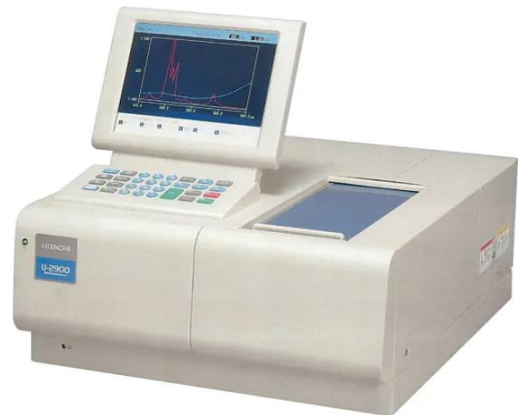
Figure 15: U-2900 UV-visible spectrophotometer (Hitachi Ltd.)
